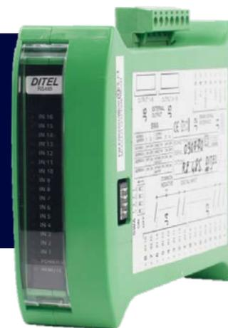
**DITEL** is an electronic module capable of extending the number of digital Input/Output of Mecc Alte controllers.
